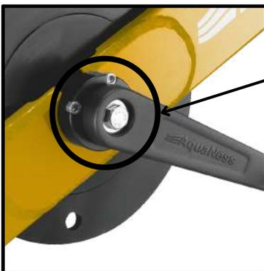
1 - Unscrew the nut on the central axle
